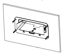
**4.** Snap the bezel onto the housing.
