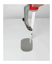
2. Insert the light into the hole and screw in using stainless steel screws.
