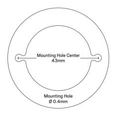
Using 1:1 mounting template or "O" ring bracket to mark the location on a surface where you want to mount the light.
